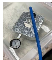
Figure 3. Safety Pressure Test
