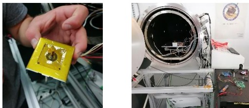
Figure 7. Electronics Vacuum Test
