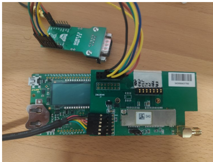
Figure 3.12. Wiring between TD1204 EVB and MCP2517 FD. Source: Own.
