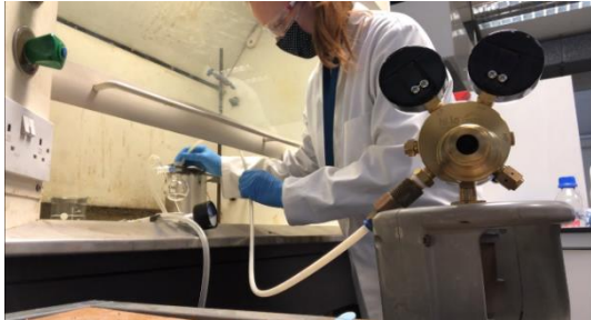
Figure 4: Nitrogen gas is bubbled through the ethanol to displace any remaining oxygen.
