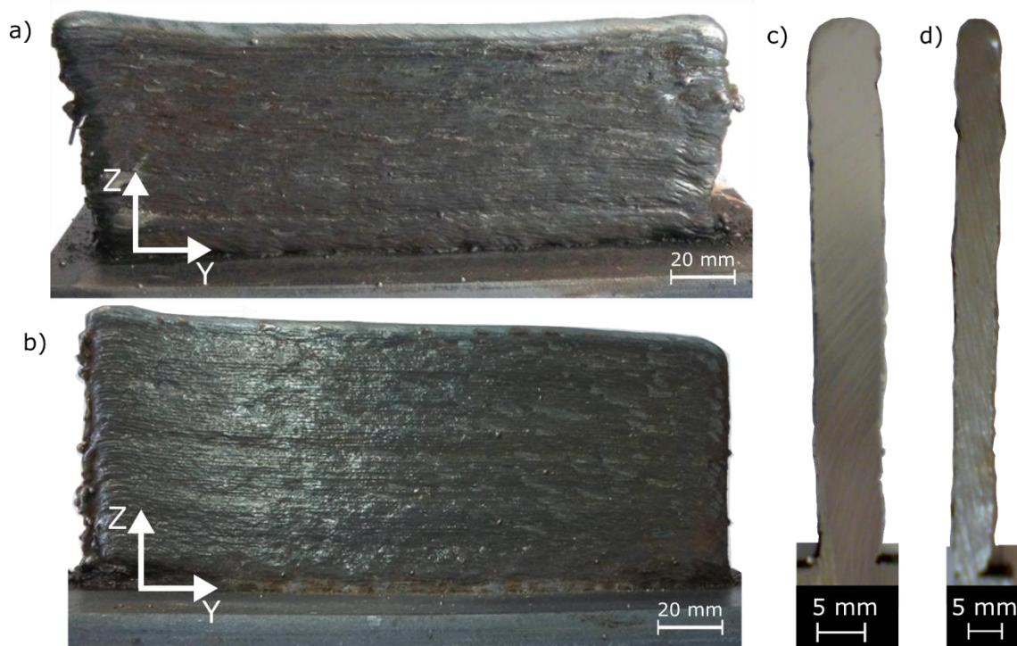
178 Figure 4 – Aspects of produced parts: a) sample P1 (high heat input); b) sample P2 (low heat 179 input). Corresponding transverse sections: c) sample P1; d) sample P2.
