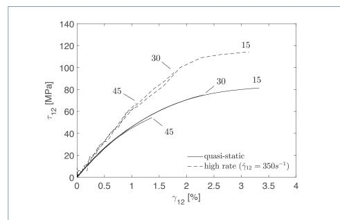
Figure 4 In-plane shear behavior derived from off-axis tension tests (engineering stress-strain curves shown).
