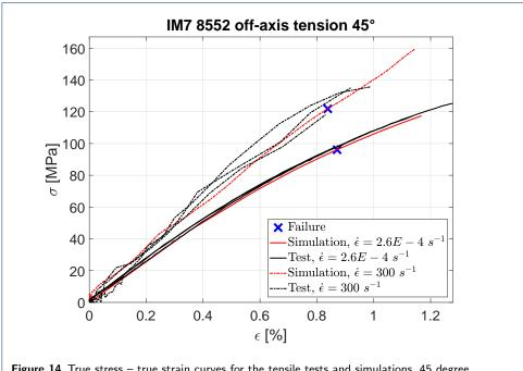
Figure 14 True stress - true strain curves for the tensile tests and simulations, 45 degree.
