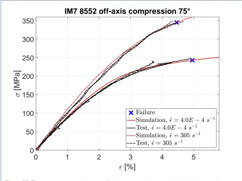
Figure 20 True stress – true strain curves for the compression tests and simulations, 75 degree.
