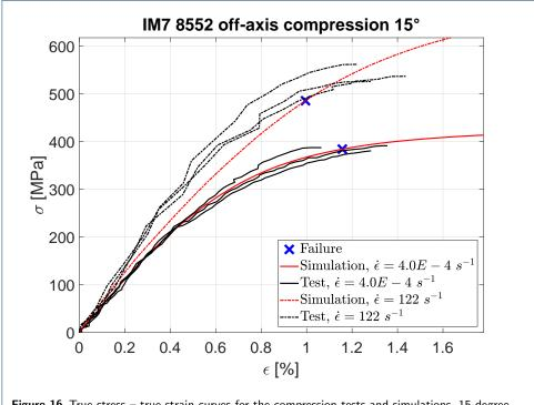
Figure 16 True stress - true strain curves for the compression tests and simulations, 15 degree.
