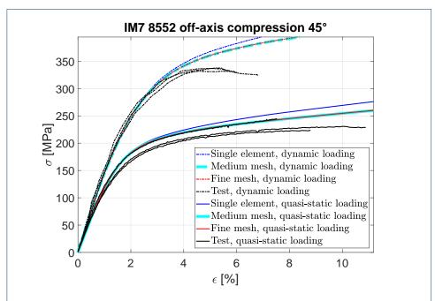
Figure 10 Comparison of the axial stress/strain prediction using different meshes during dynamic and quasi-static simulations.
