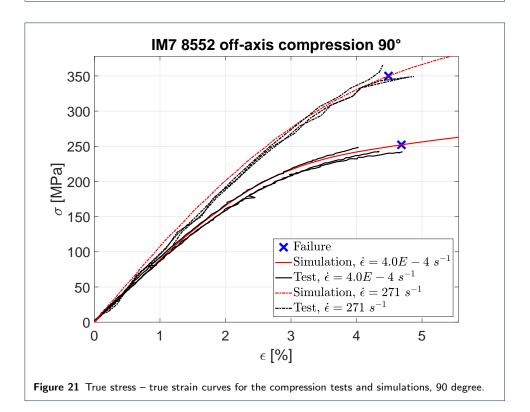
the constitutive model was well achieved for all specimen types and for both strain rate regimes. A shift from nonlinear to predominantly linear stress-strain response was observed for the dynamic off-axis tensile tests. However, the importance of Koerber et al. Page 25 of 28
