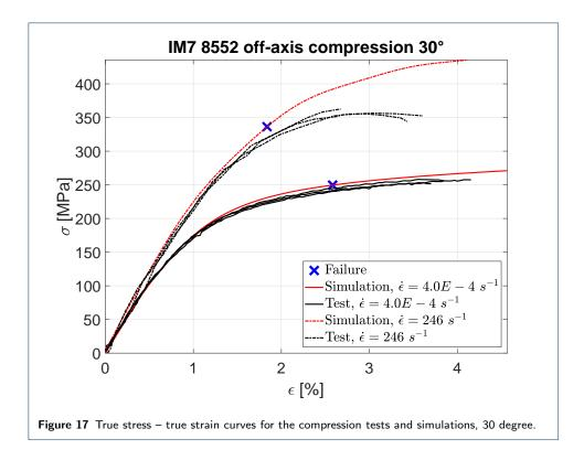
Invariant based Quadratic failure Criterion (IQC) based on the work of Vogler and co-workers [11, 24] was implemented. The model provides good predictions of the stress-strain state, regardless of the size of the finite elements, meaning that using Koerber et al. Page 23 of 28
