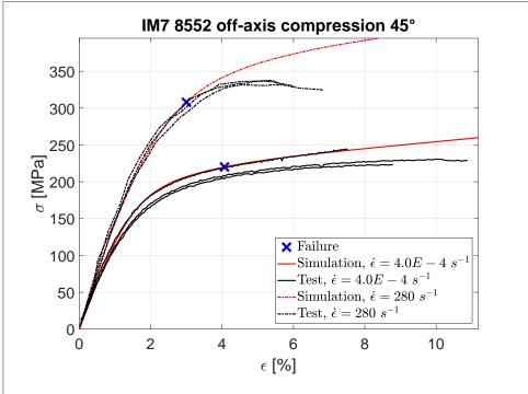
Figure 18 True stress - true strain curves for the compression tests and simulations, 45 degree.
