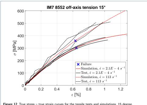
Figure 12 True stress - true strain curves for the tensile tests and simulations, 15 degree.
