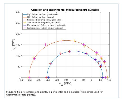
The IQC uses the same formulation as the yield criterion for the matrix failure which lead to similar shaped yield and failure surface. In the Section Results are shown the failure points simulated on stress-strain diagrams the further described meshes.
