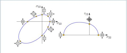
Figure 5 Schematic representation of the yield surface for UD composites in stress space.
