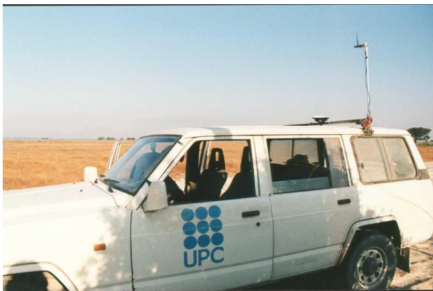
Figure 7. Top: receiver and radio link at RTK “base”. Bottom: “Rover” vehicle, with the GPS and the radio antennas at the roof.
