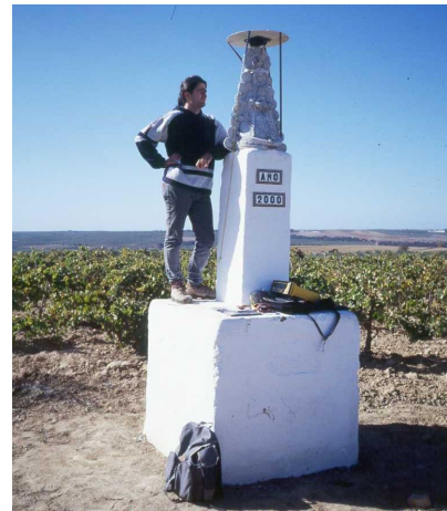
Figure 2. a) Geodetic Network established for the project. b) Example of geodetic point (Retamales), used to link the local network with REGENTE, (IGN)
