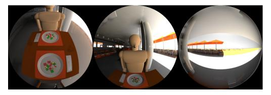
**Figure 3.** Simulated pictures of Sal Café restaurant with each workplane: table, a person in front and window.
