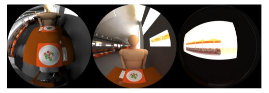
**Figure 8.** Simulated pictures of window façade system of Sal Café restaurant with each workplane; table, a person in front and window.
