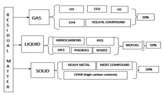
Fig. 4 Matter resulting from the Pyrolysis process [10]
