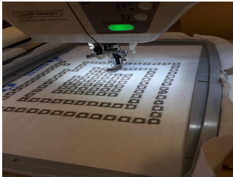
Figure 9. Process of embroidering the square FSS embroidery structure.
