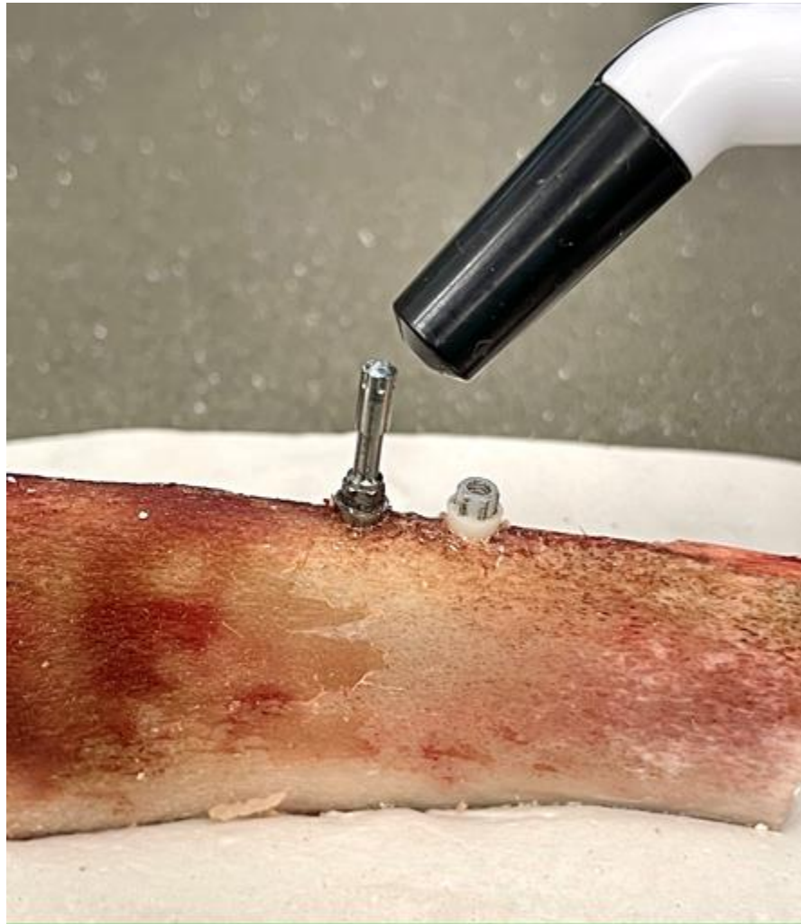
Figure 3. Measurement of implant stability by resonance frequency analysis using a Penguin and its Multipeg transducer screwed to the Ti implant, expressed in ISQ values. On the right, the Zr implant placed in the same rib can be seen.
