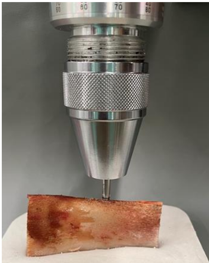
Figure 2. Placement of the implant, in the surgically shaped bone bed, using a calibrated torque meter, to record the insertion torque in Ncm.
