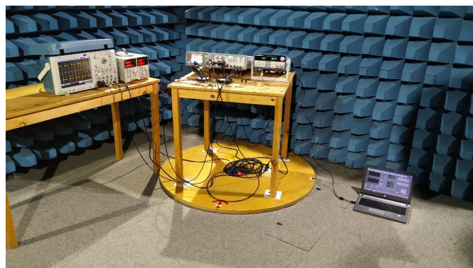
Fig. 9. Measurement setup for characterisation of the power losses of the EPC2001C.
