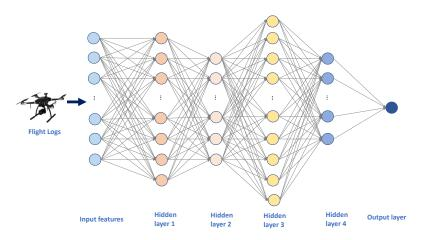
Fig. 3. An MLP for GPS spoofing attack detection.
