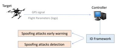
Fig. 2. Illustration of our proposed solution for synchronous spoofing attack detection and prevention; it involves a flight controller, a communication channel between the target and the controller, and a software intrusion detection framework (DNN-based).
