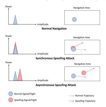
Fig. 1. Synchronous versus asynchronous spoofing attacks.
