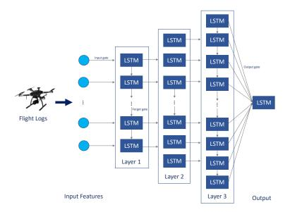
Fig. 4. An LSTM model for GPS spoofing attack detection.
