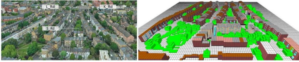
Figure 16 Left: Aerial view of the case study area and corresponding detailed ENVI-met model. Right: view of the physical model and corresponding simplified ENVI-met model (2 columns picture)
