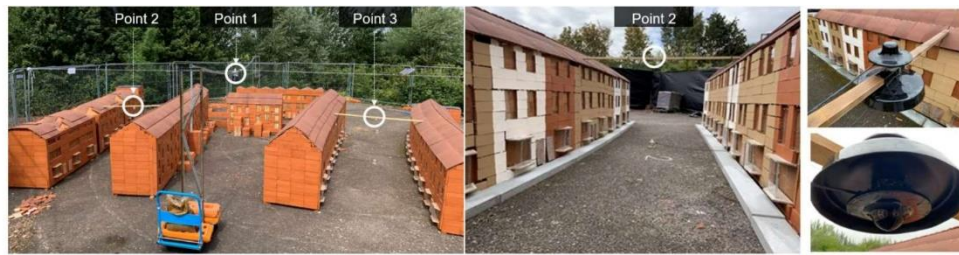
243 Figure 3 Views of the 1:10 physical model of the case study area before and after the application the façade colours and 244 details of the pyranometers installed. The circles indicate the location of the pyranometers (2 columns picture)
