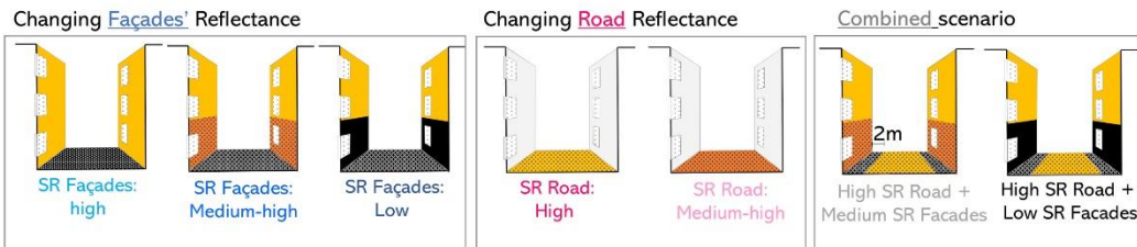
286 Figure 4 Simulated scenarios with varying solar reflectance (SR) of the façades' and road' materials (2 columns picture)
