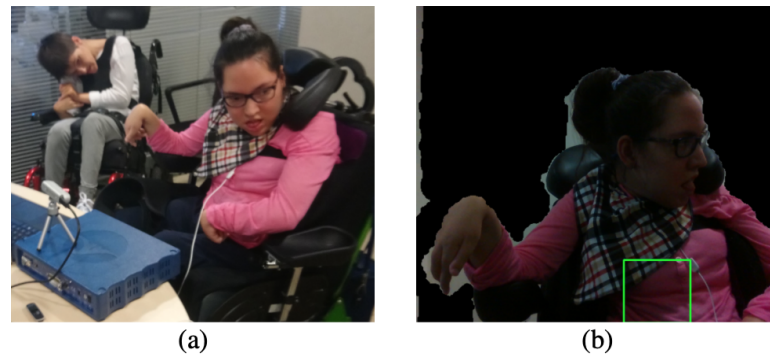
Figure 5. (a) Acquisition in a healthcare environment with a disabled user showing a non-standard pose. (b) Computer view during the execution of the proposed algorithm. The masked background could be observed as well as the ROI, which is marked in green.
