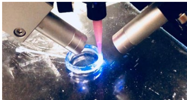
Figure 3. Light Curing system with two UV-Led's.
