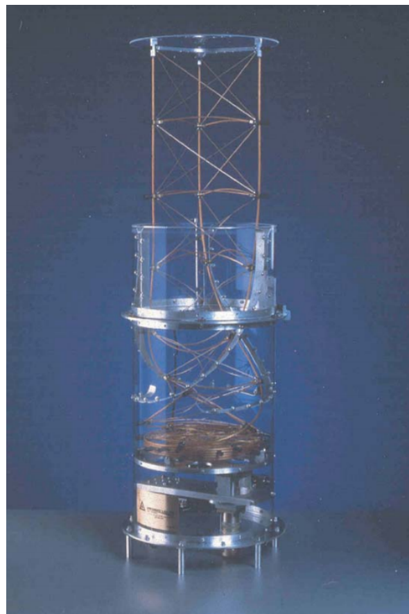
FIGURE 1.4: Coilable mast concept (left) [34] and application inside a canister and deployed through a rotating nut (right) [30]
