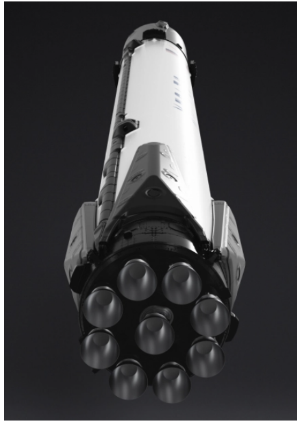
Figure 8: Falcon 9 first stage octaweb engines [7]
