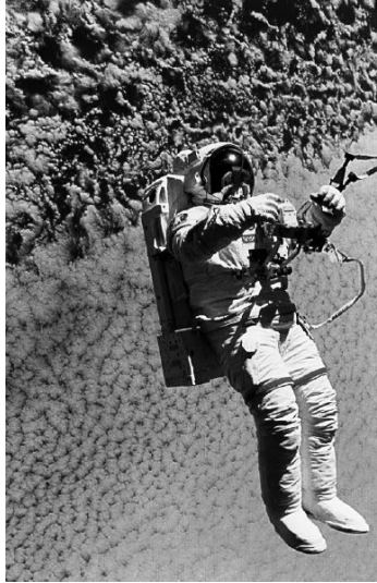
(Fig. 2.13.: Mark C. Lee test flies the Simplified Aid for Extravehicular activity Rescue (SAFER) device during the STS-64 mission)
