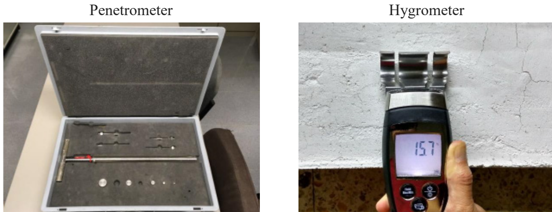
Fig. 2 NDT portable devices used in this study Source: authors
