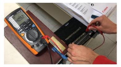
Figure 4. Strain sensor characterisation setup.
