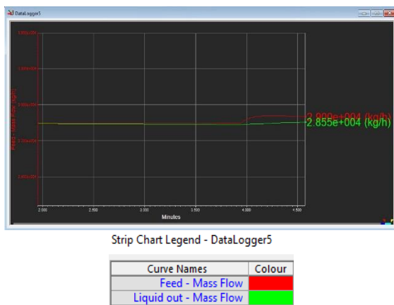
Figure 16. Datalogger 5 evolution after the change in pressure from 390 kPa to 420 kPa on the Feed.
