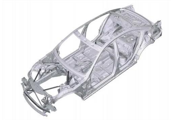
Figure 22. Monocoque chassis. (Source: (Rangam Kartik, 2020) Types Of Car Chassis Explained | From Ladder To Monocoque )
