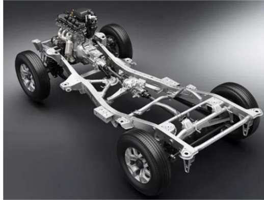
Figure 18. Ladder frame chassis. (Source: (Rangam Kartik, 2020) Types Of Car Chassis Explained | From Ladder To Monocoque )
