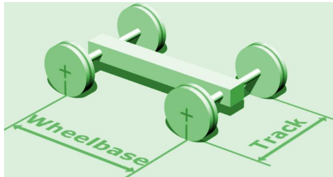
Figure 15. Wheelbase and track (Source: Wheelbase: How Important Is It In Designing The Vehicle? - CarBikeTech)
