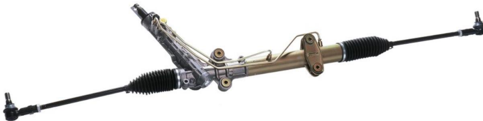
Figure 56. Rack and pinion steering system of a real car (Source: (Matt Robison, CarThrottle (2018) | What Actually Is Rack And Pinion Steering?) )
