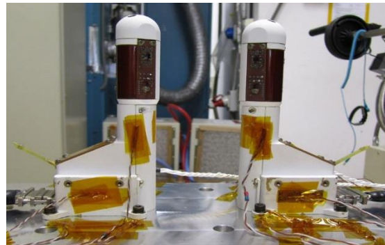
Figure 9: TWINS Booms ready to be installed. CAB/INTA-CSIC
