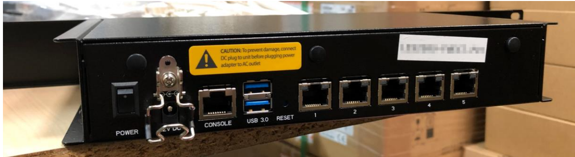
Figure 34: Firewall Barracuda F18 Revision B rear side
