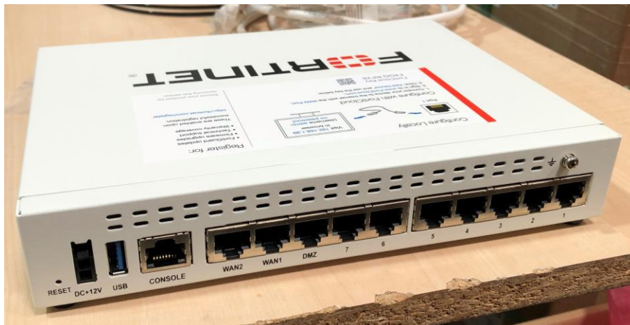
Figure 32: Fortinet's rear side
