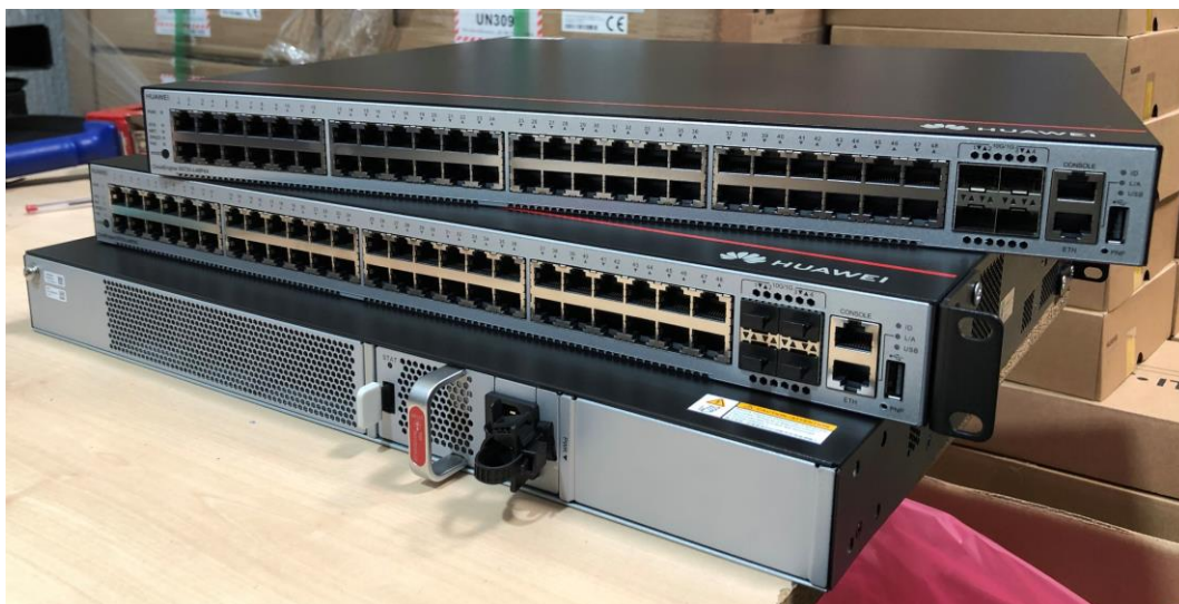
Figure 30: 3 switches Huawei S5735-L48P4X-A
