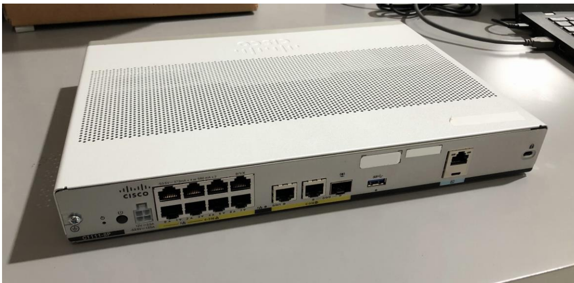
Figure 3: Router Cisco C1111-8P
