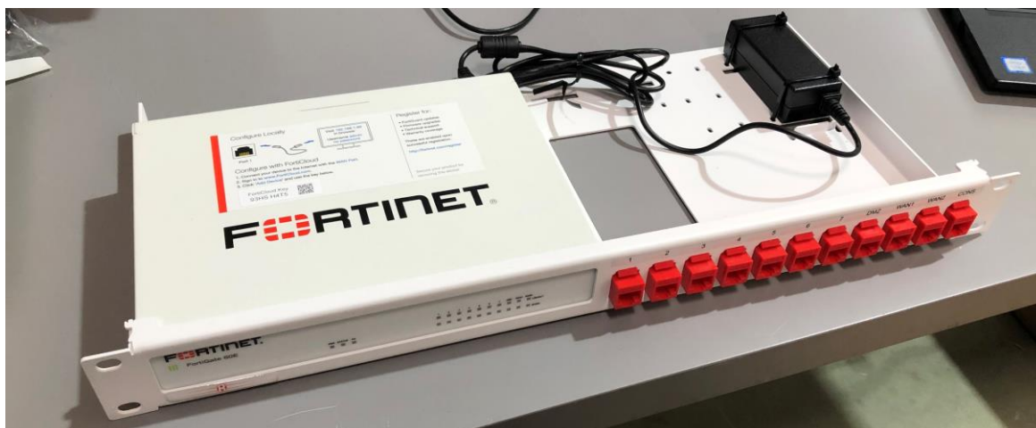
Figure 33: Fortinet adapted to rack size standards
