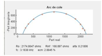
Figure 4.9: Cole-Cole function applied to an apple
