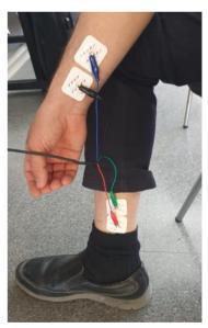
Figure 4.10: Static body -Electrodes placement
