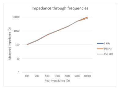
Figure 4.2: Impedance in different frequencies
