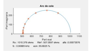
Figure 4.5: Cole-Cole arc with RC net
