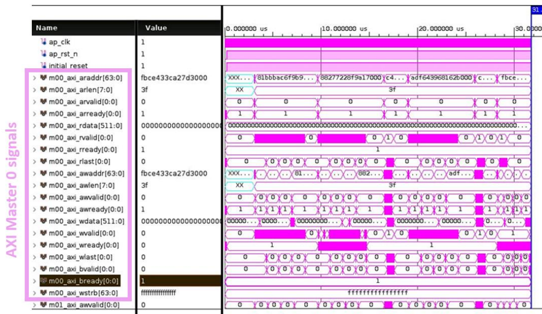
Figure 32. AXI Master 0 interface signals in Vivado Simulation.
