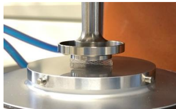
Figure 25. Compression test of the stents.
