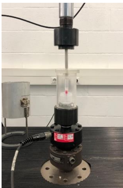
Figure 21. Injectability test setup.
