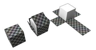
Figure 2.4: Representation of the UV mapping/unwrapping of a cube. Source: [58]
