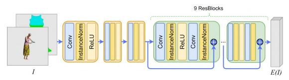
Figure 4.5: Parameter-Sharing Encoder architecture. Contains three convolution blocks and nine residual blocks. Source: Own elaboration.
