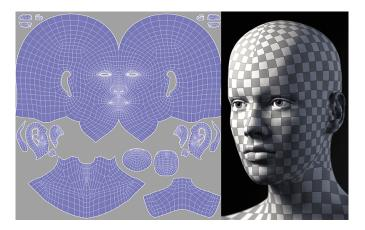
Figure 2.3: Example of a 3D face model and its corresponding UV map. Source: [58]
