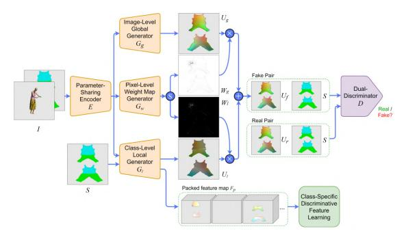
Figure 4.3: Overview of the proposed LGGAN. The symbol  $\oplus$  denotes element-wise addition,  $\otimes$  element-wise multiplication and  $\otimes$  channel-wise softmax. Source: Own elaboration adapted from [56].
