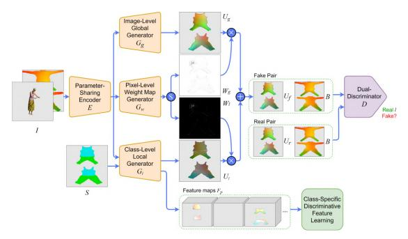
Figure 4.4: Overview of the proposed LGGAN when conditioning also on SMPL body UV map B. The symbol  $\oplus$  denotes element-wise addition,  $\otimes$  element-wise multiplication and  $\otimes$  channel-wise softmax. Source: Own elaboration adapted from [56].
