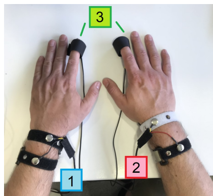
Fig. 5.7.: Measurements on a patient. Signals acquired: 1. ECG; 2. IPG; 3. Tonometer 1 and 2.
