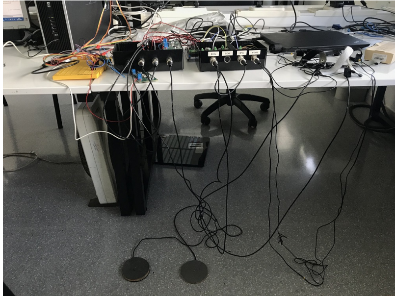
Fig. 3.7.: Different front-end devices developed by the research group, used to acquire different biosignals.
