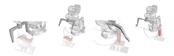
The elaborated script to develop the robotic path through the ruled surface was given to students at the beginning of the session. In this case, the geometry input is a ruled surface in which, as mentioned previously, a specific set of planes were extracted and then sent to the robot (Fig.14)
