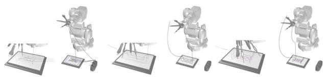
Fig. 13. Images of the robotic path programming characterization for the dripping operation, for the awl manipulation type 1, and for the awl manipulation type 2.
