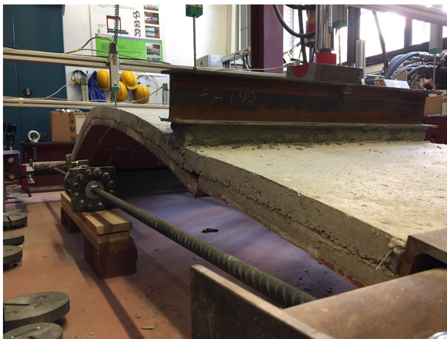
Fig. 8. Composite vault 1 showing two hinges and its failure mechanism.
