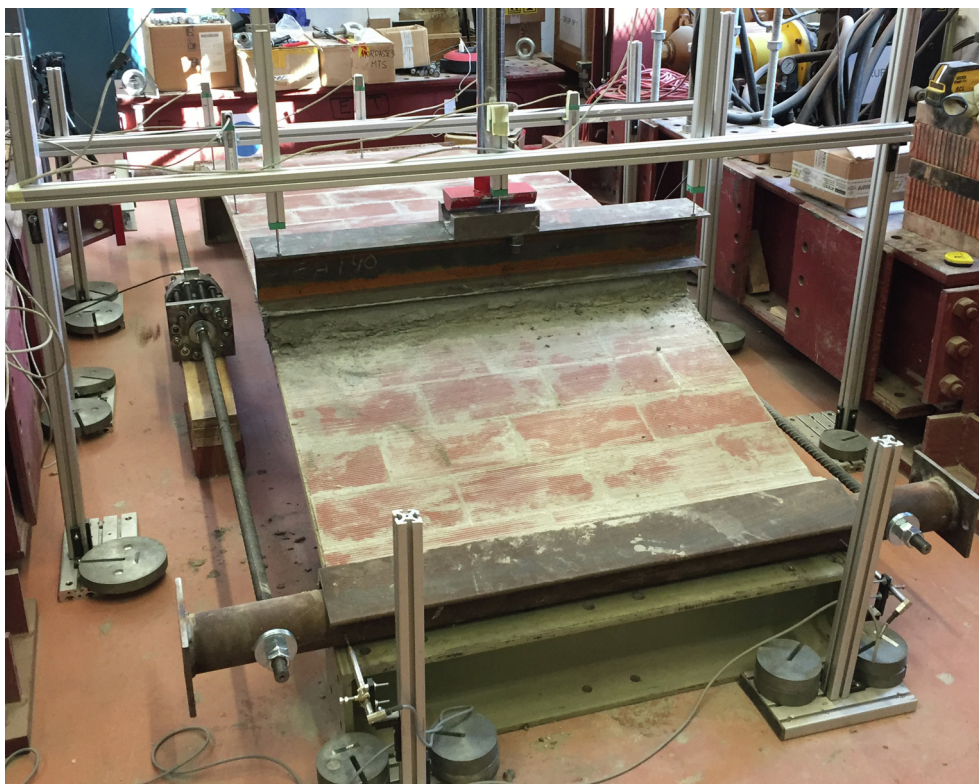
Fig. 19. Load test setup of the plain, unreinforced, tile vaults.
