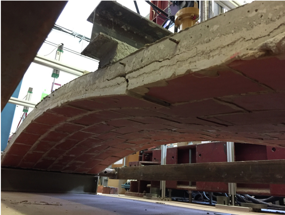
Fig. 24. Formation of the hinge under the load. Composite barrel vault 4.
