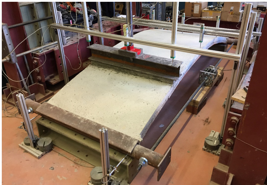
Fig. 6. Load test setup of the tile-concrete composite vaults.
