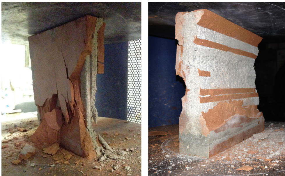
Fig. 3. Compression tests on tiles. Left) extrusion direction, right) orthogonal direction.
