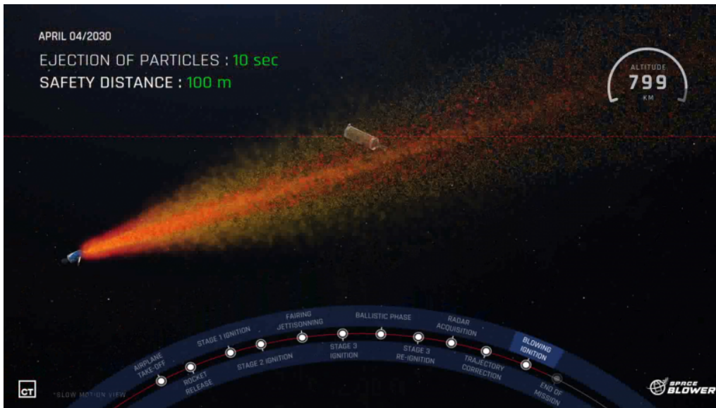
Figure 2.5: CNES' Spaceblower ejecting particles to deviate the debris' trajectory [24]
