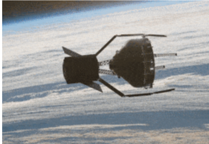
Figure 2.4: ClearSpace-1 simulation where it captures Vega's payload adapter [23]
