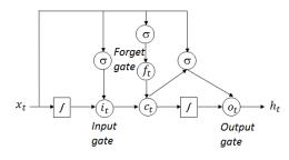
Fig. 6. LSTM Memory Cell structure.
