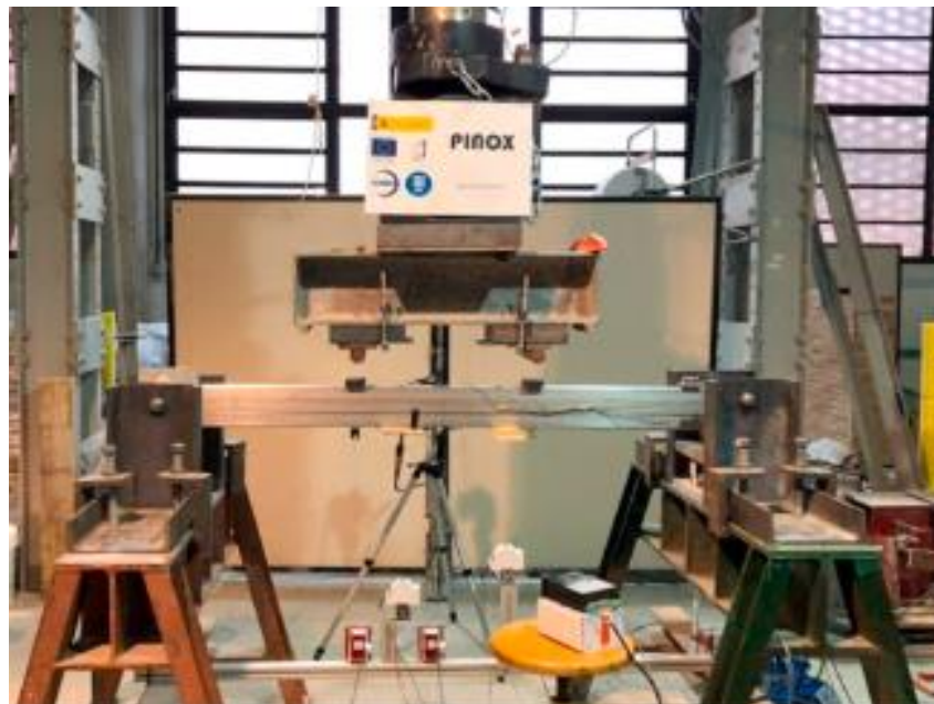
Figura 3.2. Esquema "Four Point Bending Test" (Arrayago et al., 2020)
