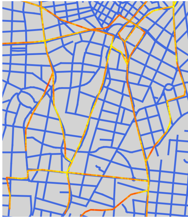
Figure 6: Heatmap of Athens small. 5000 seeds used on the reconstructed map with a radius of 75m. Each one is colored according to its F-score. The brighter the color (yellow), the more accurate the region of the reconstructed map.
