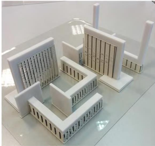
Figure 2.7 Different support material in different printing orientation [21]
