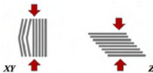
Figure 2.14 Scheme of the compression force influence on the layer direction [22]
