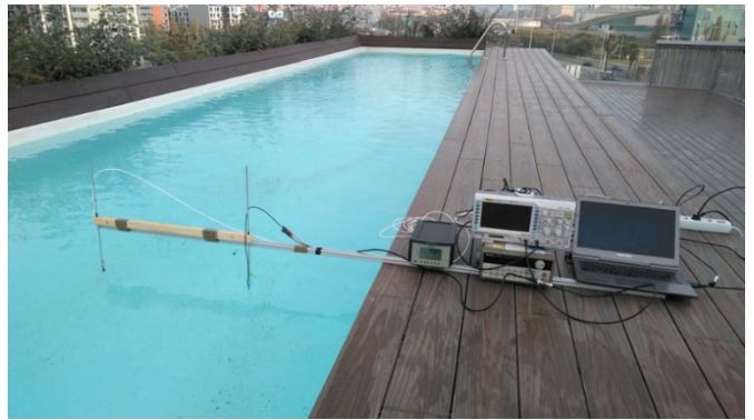
Fig. 6. Test tank of 2.5x14x1.5 m in dimension with a Brüel & Kjaer hydrophone (left) and a piezoelectric transducer under test (right), and the amplifier, signal generator, oscilloscope and computer used to conduct the measurements.
