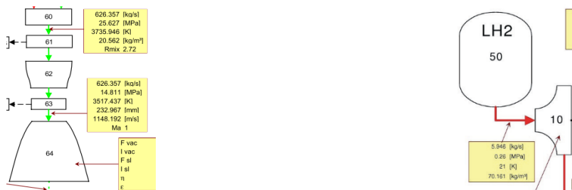
(a) Higher temperature in the RD-180 cycle (Fig. A.13)[1] (b) Lowest temperature in the Vinci cycle (Fig. A.9)[2]
