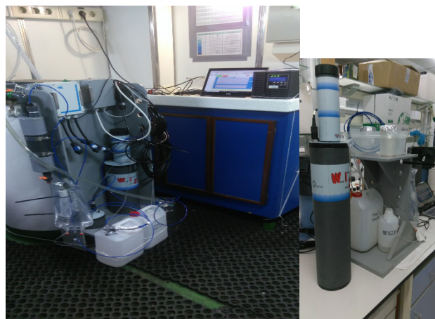
Fig 1. (a) WIZ probe-thermosalinograph-GPS module on board; (b) WIZ probe calibration in the laboratory.
