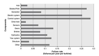
Fig. 1: Average failure rates for WT components. [4]
