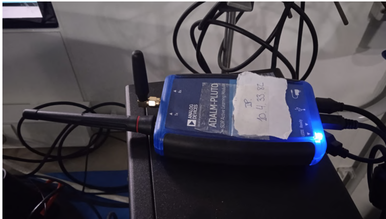
Figure 2.11: Picture of the Pluto SDR board used for the emulated ground station.
