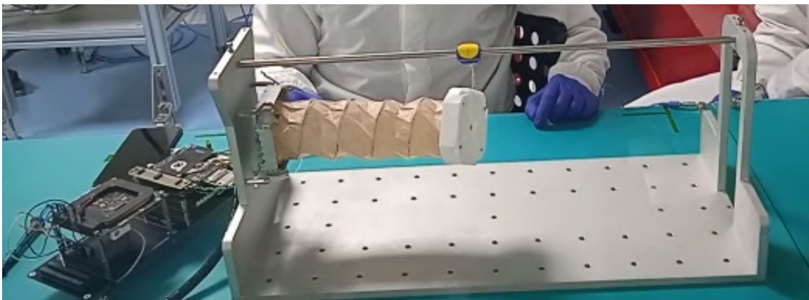
Figure 3.17: Picture of the half deployment of the NADS deployment test.
