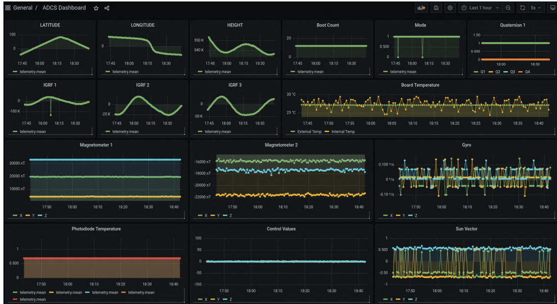
Figure 2.12: First version of the ADCS dashboard using Grafana.
