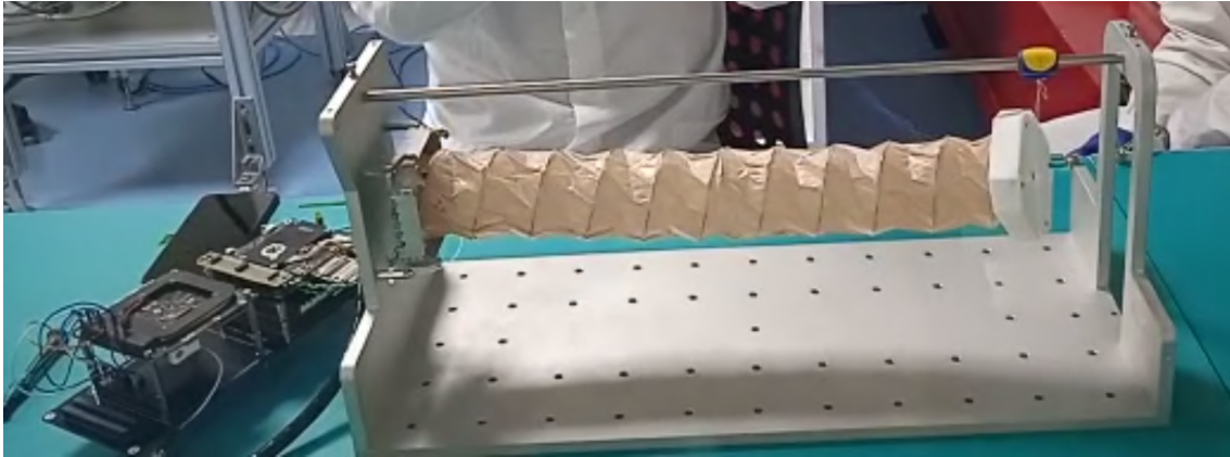
Figure 3.18: Picture of the full deployment of the NADS deployment test.
