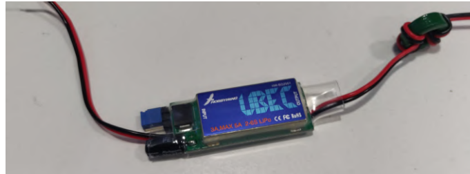
Figure 3.23: Regulator, UBEC 3A
