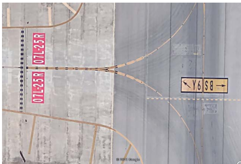
Figure 3.4. Example of taxiway markings in Barcelona–El Prat Airport. (Image captured using Google Earth).
