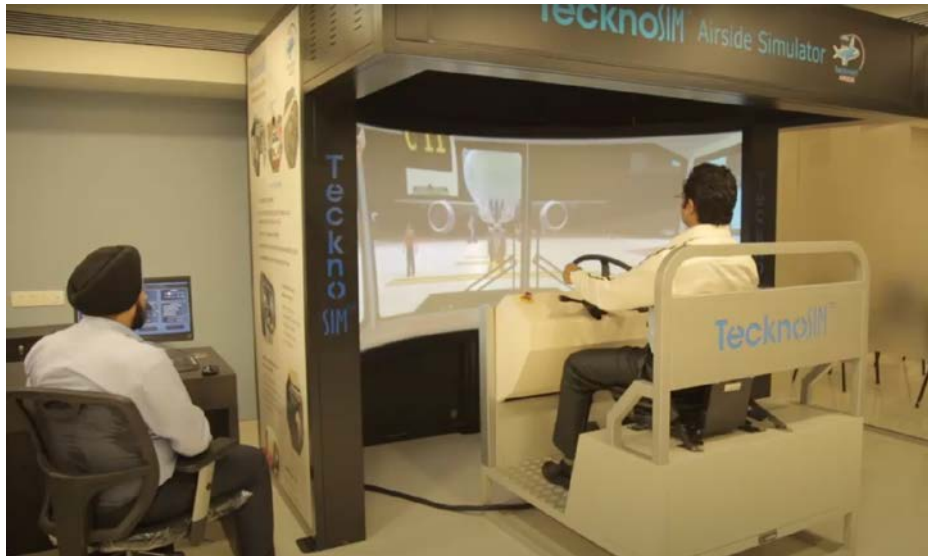
Figure 2.2. Tecknotrove System (I) Pvt Ltd. (2017). Electric motion platform and curved projection display. https://www.youtube.com/watch?v=-TzDYp65zo4 [15]
