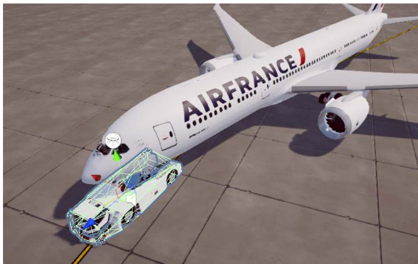
Figure 4.24. TaxiBot and Boeing 787 models connected through a hinge component.
