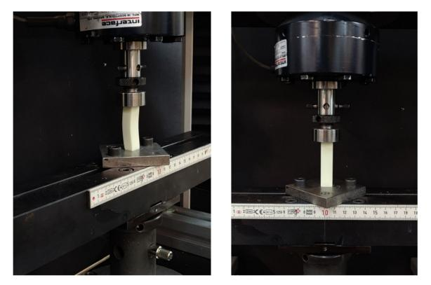
Figure 3. Experimental test set-up for reinforced compression specimens ( $12.7 \times 12.7 \times 50.4$  mm).
