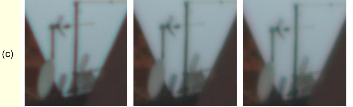
Here the results of the application of our method can be seen: (a) Reference image, (b) real images seen through the antique telescope and (c) simulated images of parabolic antennas. We obtained the simulated ones convolving the PSF of the instrument with (a). Using this method we can see the images as they would have been seen in their time without removing the instrument from the museum.
