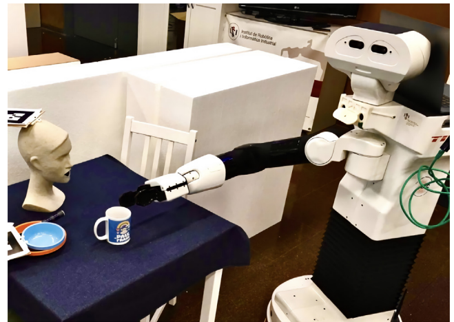
Fig. 1. TIAGo robotic platform developed by PAL Robotics performing a manipulation task.
