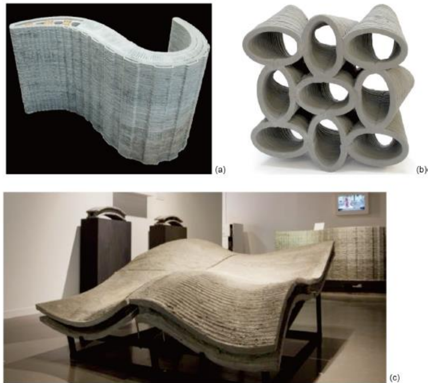
Figure 47 3D components manufactured by concrete printing. (a) Wonder bench (2 m×0.9 m×0.8 m), 2015 [61]; (b) acoustic damping wall element, 2016 [145]; (c) curved-layered construction component, 2011 [146] [103]
