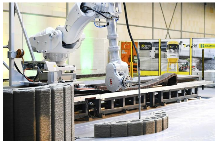
Figure 37 3D printing by Weber Beamix & BAM [59]
