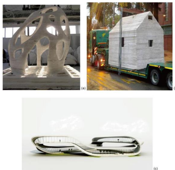
Figure 49 Largescale structures manufactured via D-shape technology. (a) 1.6 m high sculpture, 2008 [61]; (b) a complete house printed in one single process, 2010 [147]; (c) landscape house design based on a Mobius strip, 2017 [150]. [103]
