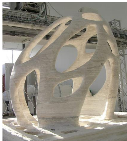
Figure 12 Radiolaria constructed by a D-Shape 3D printer [24]
