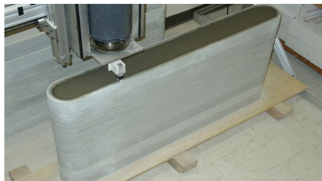
Figure 10 3D Concrete printed wall structures with conventionally cast [22]
