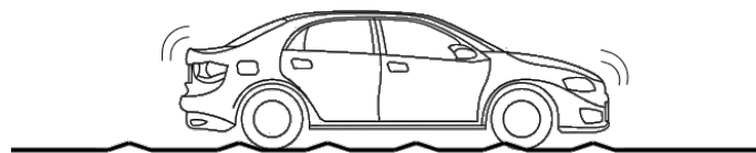
Figure 2.3: Schematic representation of a situation that can trigger the considered IMU failure mode in Table 2.2.
