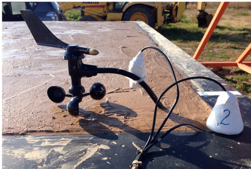
Fig. 2. Detail showing some of the external sensors and the initial conditions of the test, with the specimen's surface flush with the container's upper borders and no water film at the surface.
