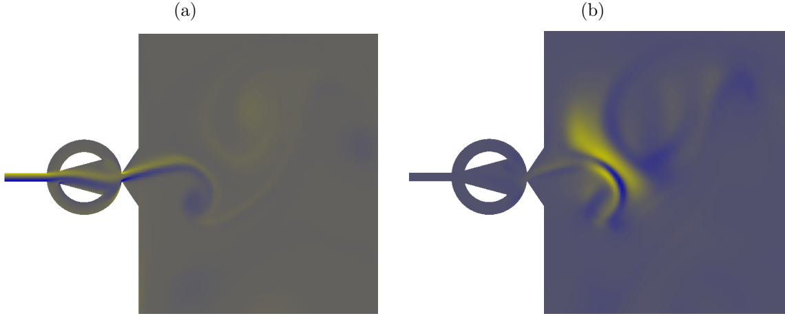
Fig. 11: Least stable pseudo-eigenmode at Re = 100 . (a) Spanwise vorticity \Omega_z \in [-5, 5] colourmap of the two-dimensional flow. (b) Cross-flow vorticity \omega_y (symmetric arbitrary range) at the same instant, well within the linear growth regime.
